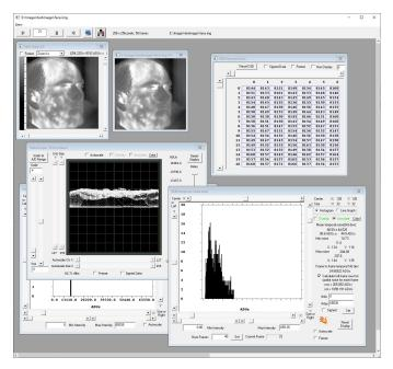
CamlRa application software showing multiple windows open to analyze images and data from an FPA.
